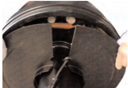
The one-piece dust cover is easily removed by releasing the worm drive clip, then opening out the two halves.
