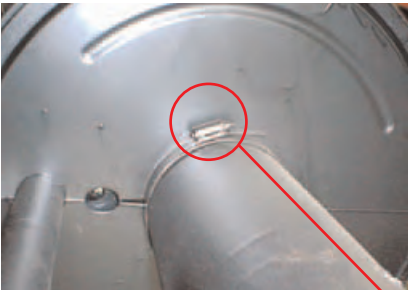
Above is a one-piece style dust cover mainly found on the 100 series axles.
