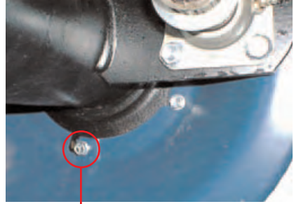
The dished dust cover is easily removed by unscrewing the retaining screws.
