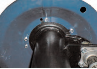
Above is a dished style dust cover found on most axle series.
